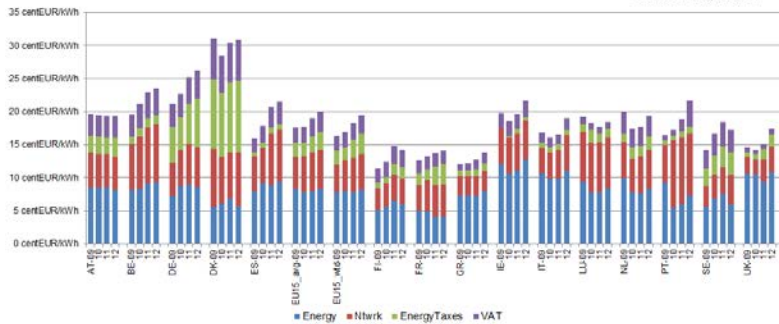
FIGURE 43 ► Retail electricity prices and their components (taxes, levies etc.) in different member states
