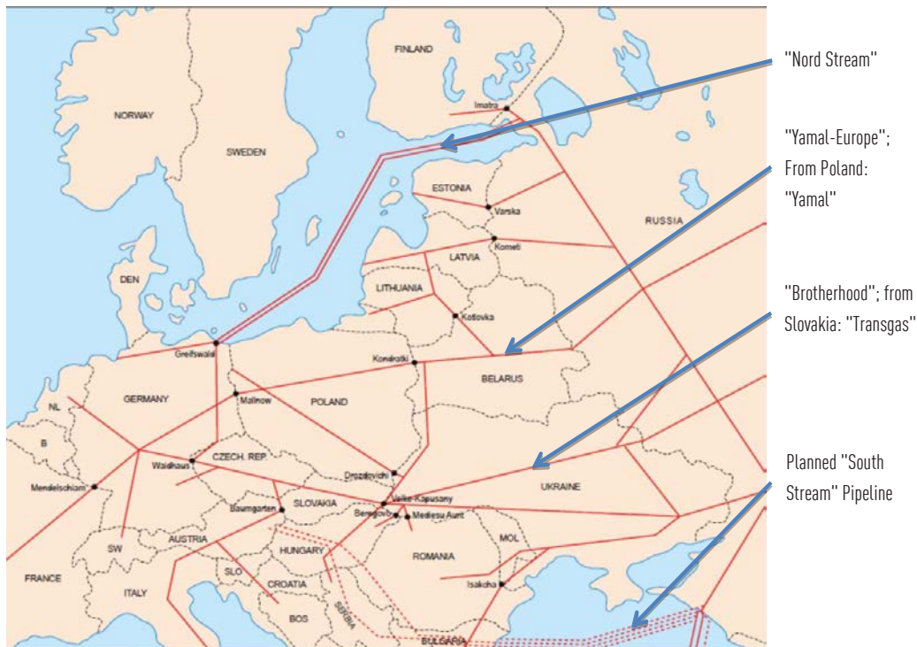
FIGURE 1 – European gas transmission network
